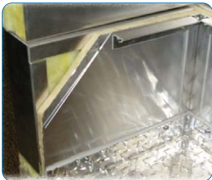
Ventrol's thermal break design with hybrid foam insulation ensures metal that is exposed to the cold side of the panel is separated from the warm equipment room side preventing condensation.
